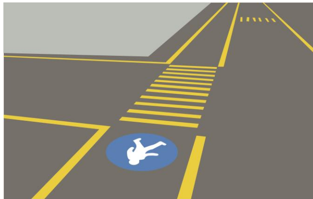
Fig.: 5.3 – Yellow Demarcation for Pedestrian Pathway
