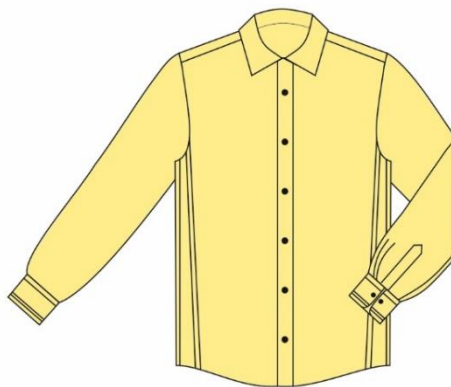
Fig.: 1.26 – Centralized placket
